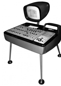
The AKAT-1 (1959) was the first differential analyzer of its kind to use transistors instead of vacuum tubes. Just as the microchip did for digital computer, this allowed for a much more compact design.
