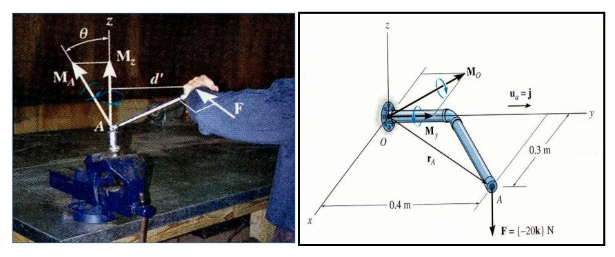
With the force F, a person is creating the moment  $M_A$ . What portion of  $M_A$  is used in turning the socket?
