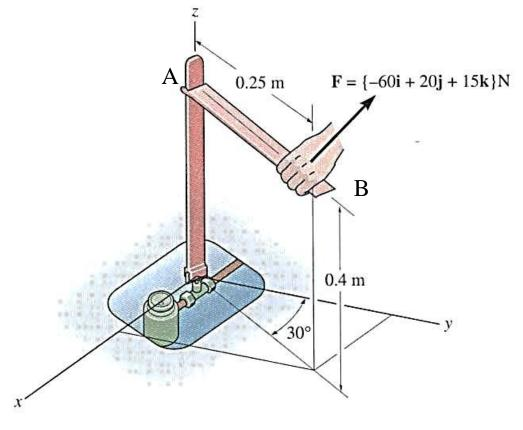
**Given:** A force is applied to the tool to open a gas valve.
