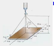
Example 3 Given: Plate has mass 150 kg Find: Tension in each cable
