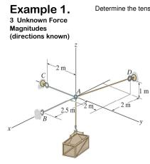
Determine the tension in cables AB, AC, and AD caused by the 600-lb crate.
