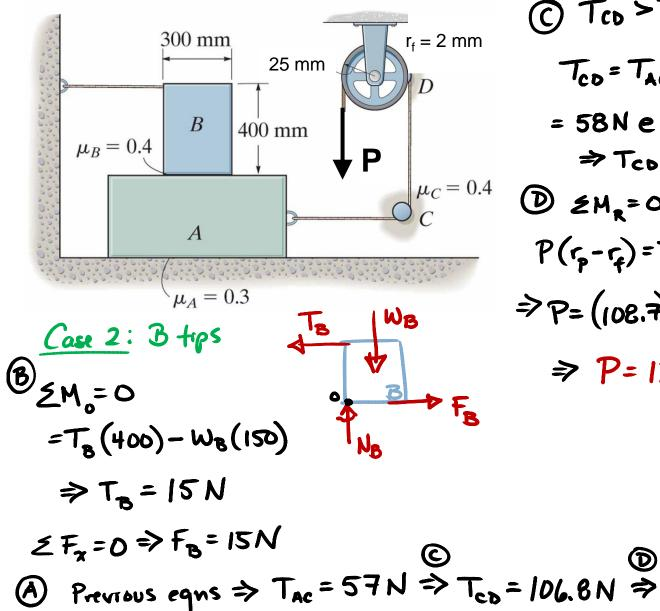
TCD > TAC Too= TAC emp = 58N e  $(0.4)(\pi/2)$ ⇒ Tco = 108.7N D ≥M,=0 >  $P(r_p - r_q) = T_{c0}(r_p + r_q)$  $\Rightarrow P = (108.7) \left( \frac{25+2}{25-2} \right)$ > P= 128 N
