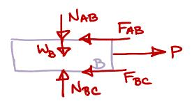
What force P is needed for motion, and will block C slide? Each block weighs 20N, and the coefficient of friction at each surface is 0.25.
