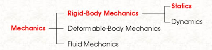
Rigid-body mechanics is further subdivided into statics, which deals with the study of rigid bodies at rest or moving at a constant velocity, and dynamics, which deals with the study of accelerated motion of rigid bodies. Statics may be considered as a special case of dynamics where the acceleration is zero, however, it is generally studied separately to ensure a firm grasp of the concepts of force, moment, and physical-mathematical modeling necessary to the study of mechanics.
