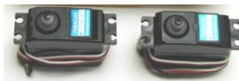
Figure 1.6: Pre-modified servos dehorned.
