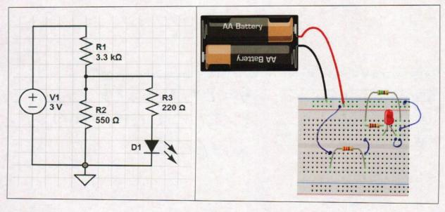
3. Rewire your breadboard from 2 so that a) the circuit still works AND b) you are measuring the current through the LED and the voltage across the 3.3 k $\Omega$  Resistor.
