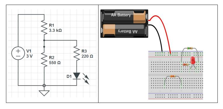
3. Rewire your breadboard from 2 so that a) the circuit still works AND b) you are measuring the current through the LED and the voltage across the  $3.3~k\Omega$  Resistor.
