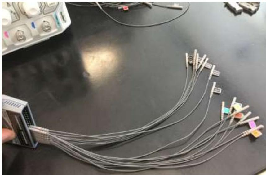
Fig. 13. Plug wires into the Logic Analyzer pins
