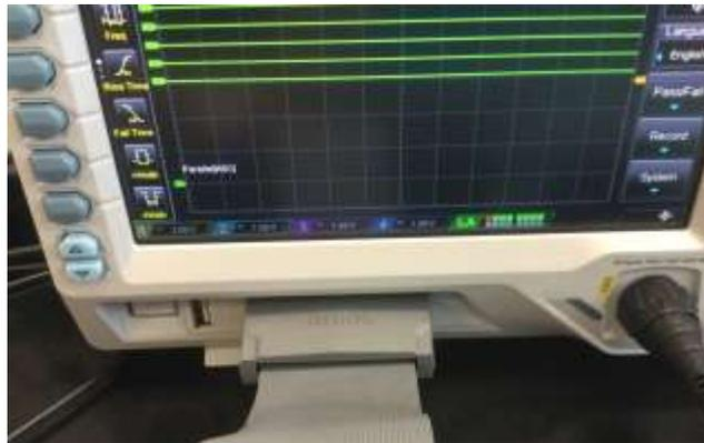
Fig. 12. Connect this connector to the scope's logic analyzer.
