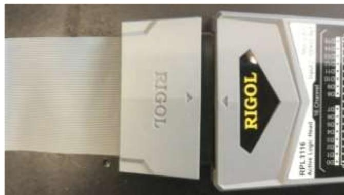
Fig. 11. Rigol Logic Analyzer Connector
