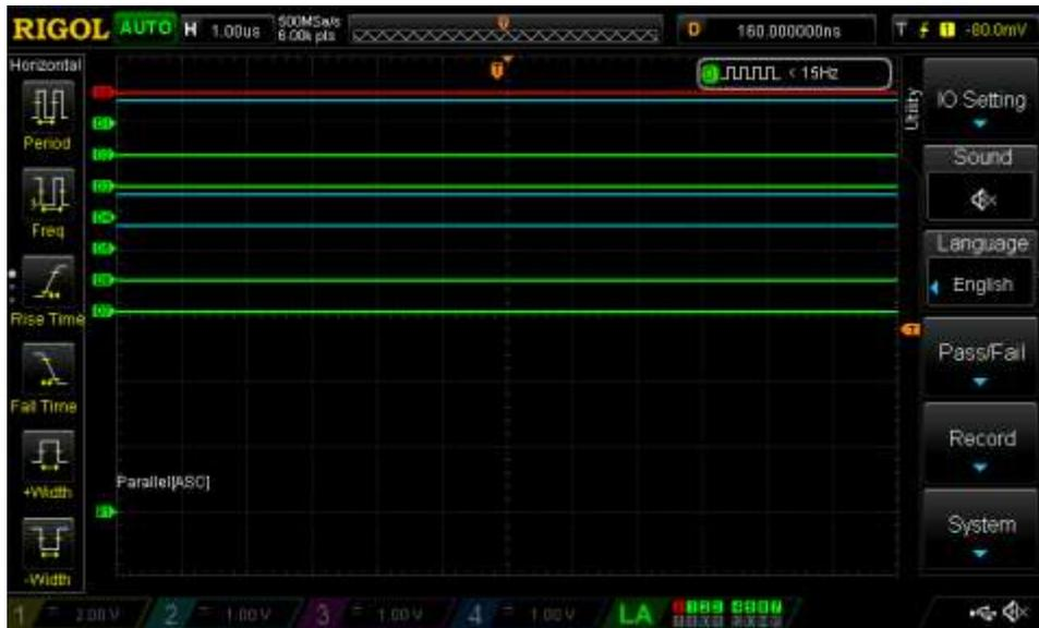
Fig. 17. State of the system with input=1V, output is "00110010".
