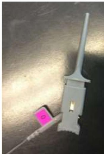
Fig. 14. Connect each labeled wire to this connector to probe the breadboard.
