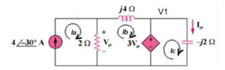
Nodal Analysis – If you examine the V1 node voltage you should be able to find a way to express that voltage in terms of Vo. Then you can set up one node equation with one unknown (Vo) to solve, and you won't need a matrix, just algebra to solve for Vo and from that you can derive Io.
