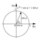
In the previous equation  $V_m e^{j\varphi}$  is a complex number that carries the amplitude and phase angle of the original sinusoid. This complex number is the definition of the **phasor transform** of the given sinusoid. In other words, the phasor
