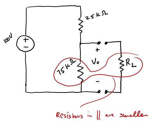
• The load "pulls down" the output voltage Not good for consumer electronics !
