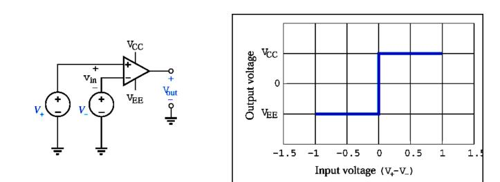
"Zero-Cross" Detector - not so good for telephone use!
