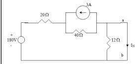
Applying source transformation to the current source yields the circuit below.
