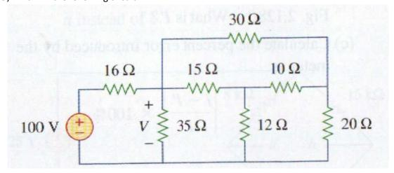
We need to find  $R_{eq}$  and apply voltage division. We first tranform the Y network to  $\Delta$  .
