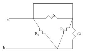
$$\begin{array}{ll} R_1//0 = 0, & R_3//5 = 40//5 = 4.444 \, \Omega \\ R_{ab} = R_2 \, / \, / (0 + 4.444) = 40 \, / \, / 4.444 = \underline{4\Omega} \end{array}$$
