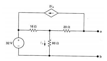
2) Now, for the same circuit above, turn off the <u>independent</u> source, connect a 1V Test power supply to terminals a-b and use the <u>mesh current method</u> to find the Thevenin Resistance. (Hint: this reduces quickly to 2 eqs, 2 unknowns that are not hard to solve. The answer for Rth is a whole number).
